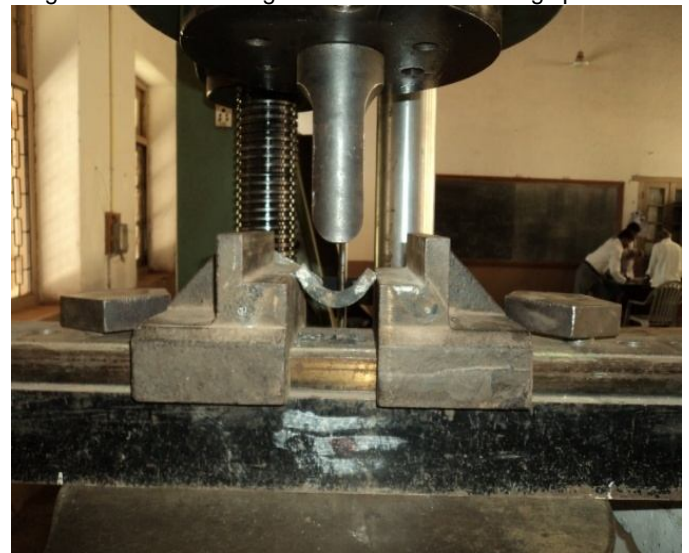
Fig. 2. Universal testing machine used for testing specimen.
